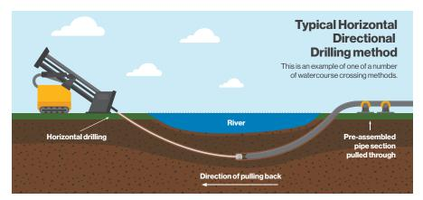
> Horizontal Directional Drilling involves drilling an underground arched tunnel when building pipelines across large rivers or sensitive crossings.
