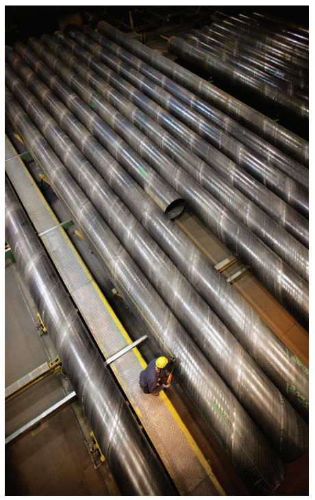
> Pipe steel is thoroughly inspected in the mill by the manufacturer using automated ultrasonic devices, and Enbridge inspectors audit those results for enhanced quality assurance.
